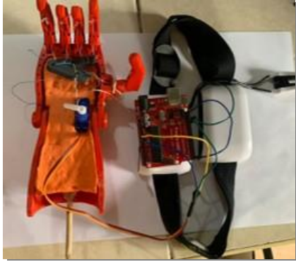
Fig. 6 Integrations of components mechanical and electrical
