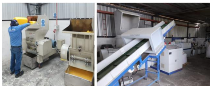
Fig. 8 PE recycling line: regrinding (left), and extrusion pelletizing (right) at Empaqplast (Quito, Ecuador). Source: Empaqplast (Personal communication)
