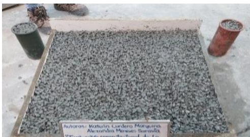
Fig. 6 Permeable rigid pavement prototype
