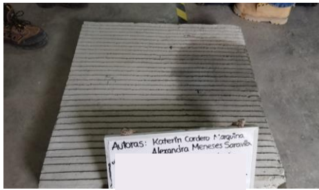
Fig. 5 Conventional rigid pavement prototype
