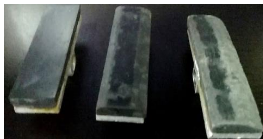
Fig. 4 Conditions or states of skid: new, semi-new and worn
