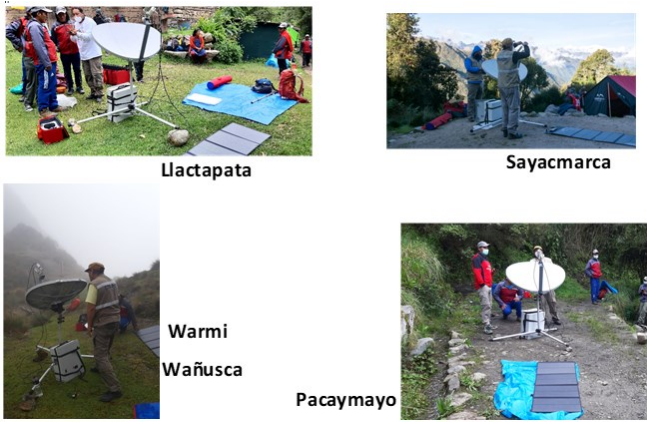
Fig. 4: Portable satellite station testing at 4 campsites along the Inca Trail Route.
