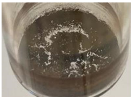
Fig 4. The solid brown is identified as C_{60}(OH)_n \cdot mH_2O .
