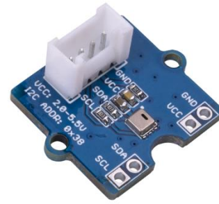
Figure 9. Grove- AHT20 I2C Industrial Grade Temperature & Humidity Sensor.
