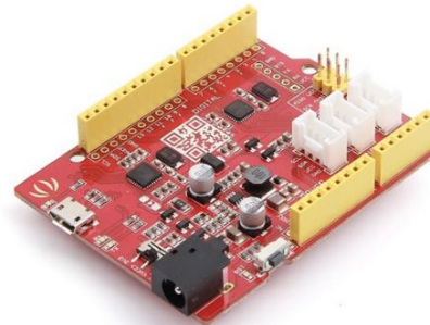
Figure 10. ATMEGA328P Seeeduno v4.2 board.
