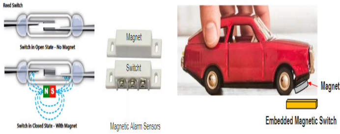
Fig. 5 Magnetic switch and sensor layout
