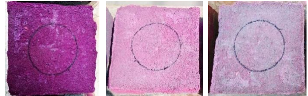
Fig. 4 Rhodamine B test - sample 4 (M-4), 0h, 4h and 26hr. Source: self-made
