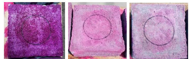
Fig. 6 Rhodamine B test - shows 9.5 (M-9.5), 0h, 4h and 26hr. Source: self-made
