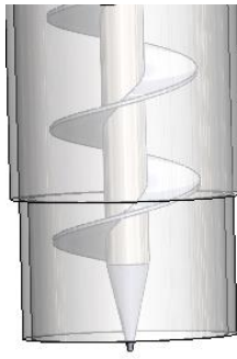
Figure 11: Updated auger drill design with drill cover
