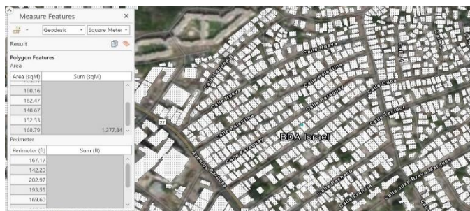
Figure 5. Israel neighborhood rooftops catchment area
