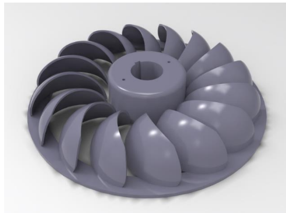
Figure 10. Buckets of Turgo Turbine
