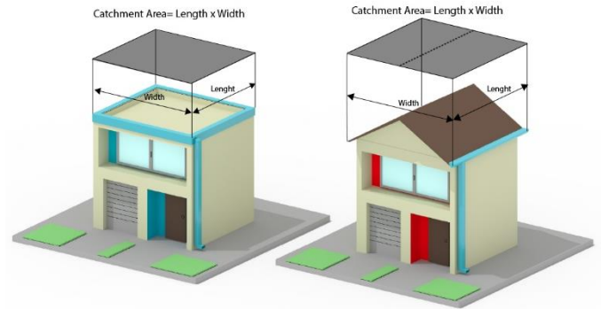
Figure 6. roofs catchment area
