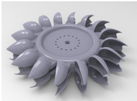
Figure 9. Buckets of Pelton Turbine
