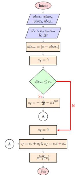
Fig. 2 Flowchart of the interaction model between a particle collision and an erythrocyte.
