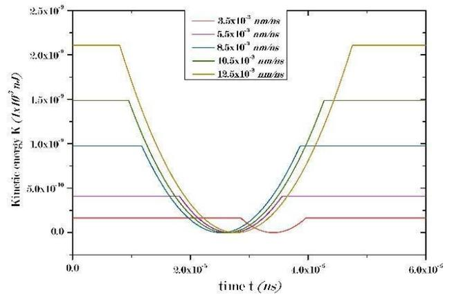
Fig. 4 Kinetic energy in the interaction between nanoparticle and erythrocyte for a particle size of 100 nm.
