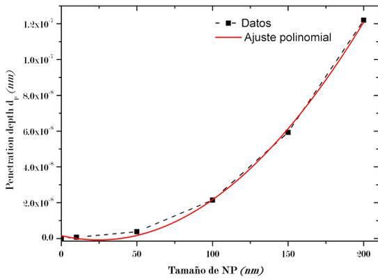
Fig. 6 Adjustment of the depth profile as a function of the MNP size..
