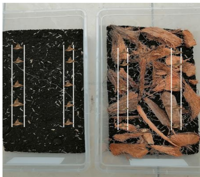
Figure 5. Set-up with biochar treatment and coconut fiber as biomantle with control set-up, showing the distribution of seedsowing in both cases.
