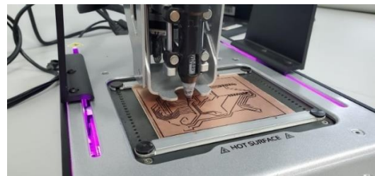
Figure 6. Adapted Voltera working with Permanent Marker.
