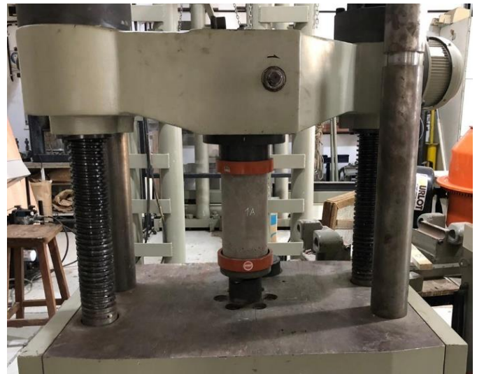
Figure 2. Compression testing in 1000 kN Shimadzu Universal Testing machine.
