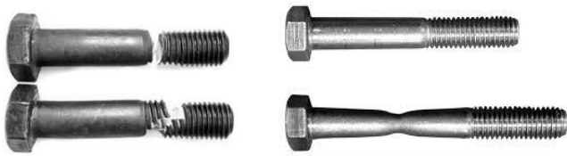
Fig.5 Bolt Fracture [8] (left), Plastic Deformation [9] (right)
