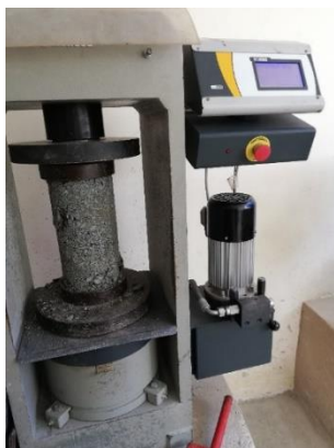
Figura 3. Specimen test machine - Compression resistance Source: Own
