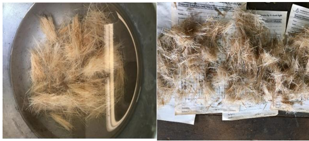
Figure 4. Saturation of Abaca vegetable fibre. Source: (Jurado Nohelia, Abril,2019)
