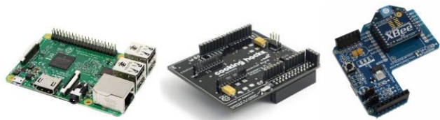
Fig. 2 Raspberry Pi 3, Connection Bridge, and Xbee Wireless Shield.
