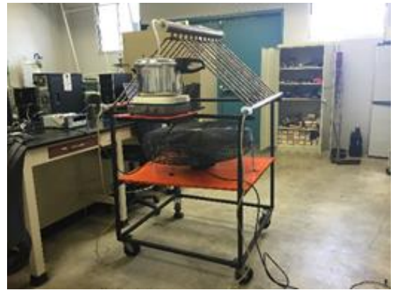
Figure 5: Actual configuration of the V-shaped ACC system
