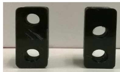
Fig. 8 On the left, first prototype, on the right chassis with modified center to center distance.
