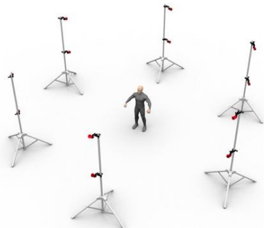
Figure 2: Example motion capture camera arrangement [15].
