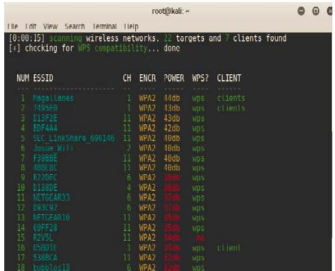
Figure 3 – Output of a typical Wifite scan
