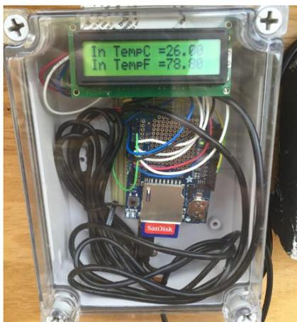
Figure 4 Arduino controller and ADAFRUIT data logging system
