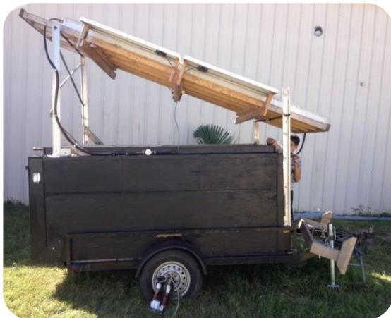
Figure 1A. Assembled Mobile Solar Digester Unit
