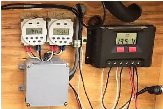
Figure 3D Battery voltage in real time
