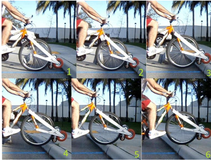
Fig. 11 Video snapshots showing BD2 hitting a 5-inch tall curb in a parking lot below 5 mph.
