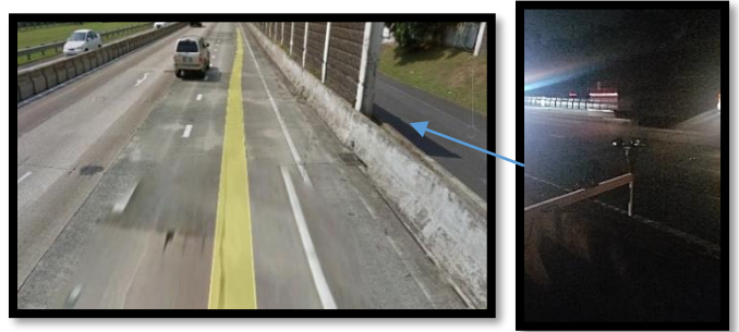
Figure 4: Anemometer set on top of barrier with an offset of 1ft at PR-52
