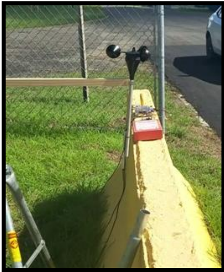
Figure 2: Experimental setup for Single-Vehicle Roadside Measurements
