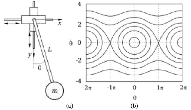
Fig. 2 Pendulum system. (a) Schematic and (b) phase diagram
