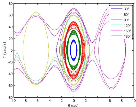
Fig. 3 Phase diagram for 1g mass with L = 1 cm
