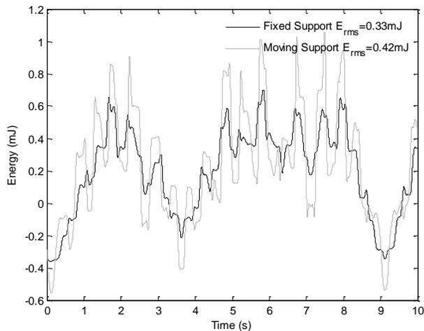
Fig. 14 Pendulum at chest ( $L = 3.7$  cm,  $m = 1$  g)
