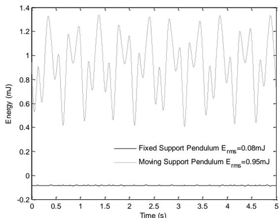
Fig. 6 Energy from a pendulum-based generator on a moving reference frame vs. a fixed reference frame
