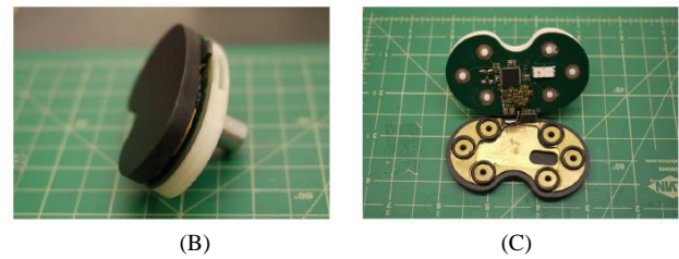
Figure 9. Images depicting the instrumented tibia with self-harvesting energy system as an assembly (A) and with the sensors grid and circuit board (B). Adapted from [85]
