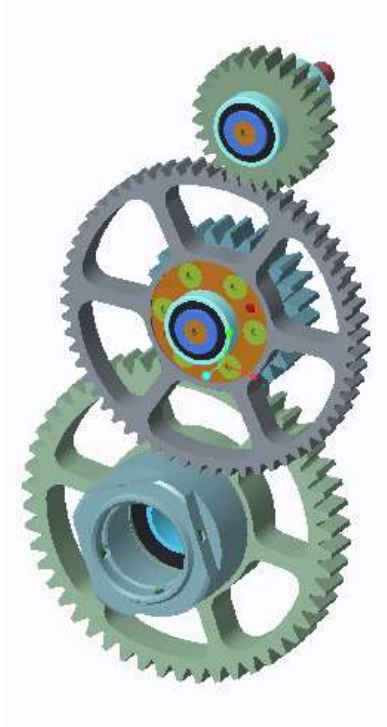
Fig. 4 Compound Spur Gear Train
