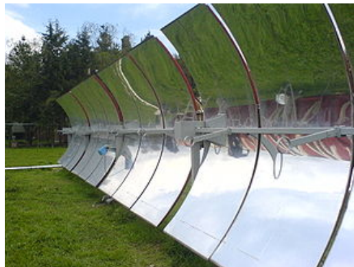
Figure 1: Cylindrical-parabolic solar collector
