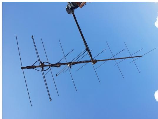
Figura 2: Antena Yagi
