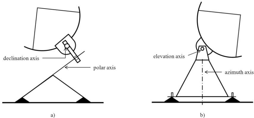
**Figure 4: Typical mounts for radio telescopes. a) equatorial mount. b) alt-azimuth mount.**
