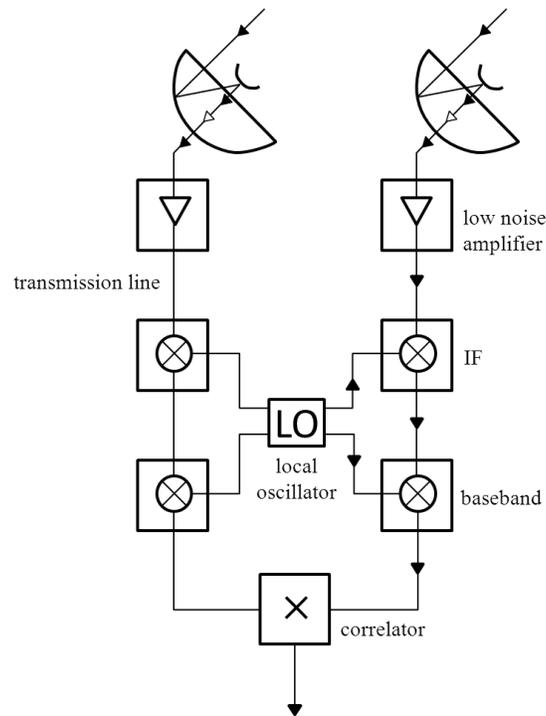
**Figure 7: Two-elements interferometry system**
