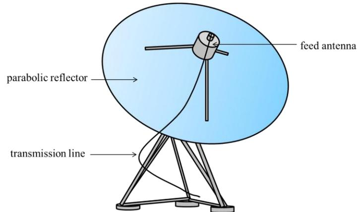
**Figure 1: Structure of a parabolic antenna**
