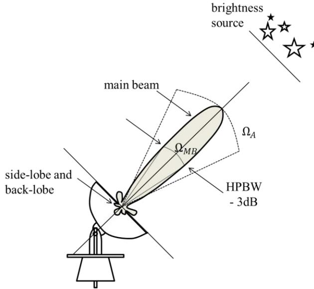
**Figure 3: Power pattern of a parabolic antenna**
