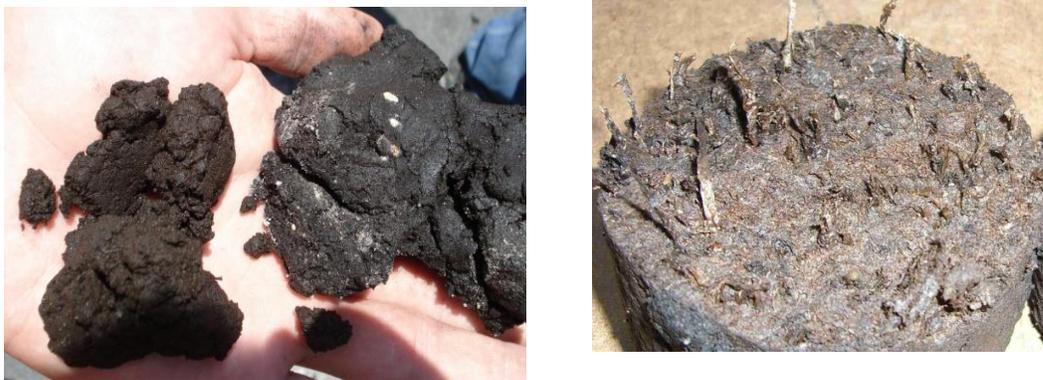
Figure 1: (a) Silty organic layer from 1.5m to 3.0m; (b) Fibrous peat layer from 3.0m to 6.0m.
