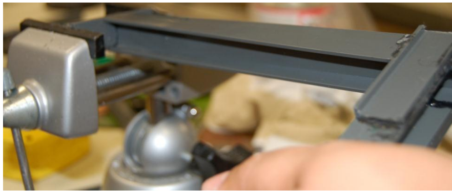
Figure 2: Torsional deformation of ABS beams and connection
