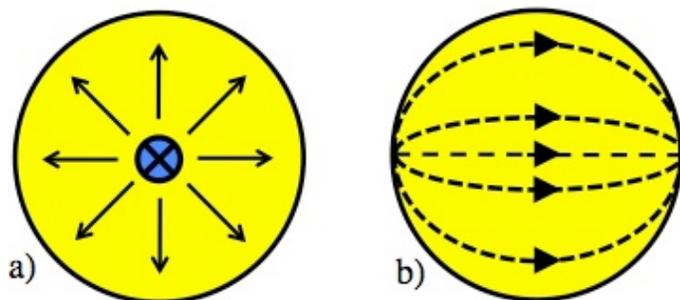
Fig. 1 Symmetric streamlines of flow over sphere. Front down stream view a) and side view with projected streamlines b).
