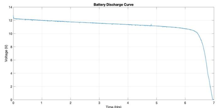
Fig. 4 Deep-cycle battery discharge curve at 0.1C
