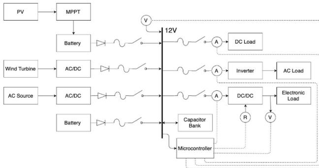
Fig. 1 Scheme of the proposed test bench.
