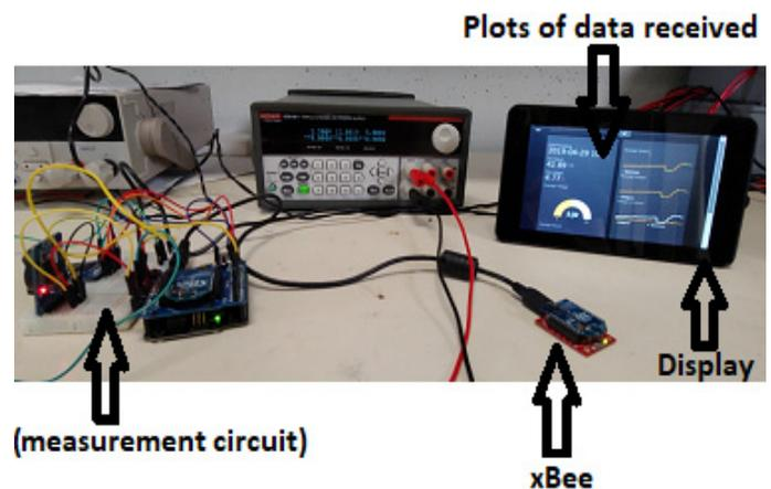
Fig. 7 Preliminary monitoring system
