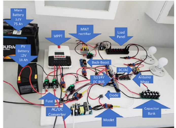
Fig. 3 Test bench implemented
