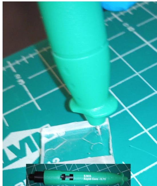
FIG. 4. Hole punching in the microchip using a biopsy punch.
