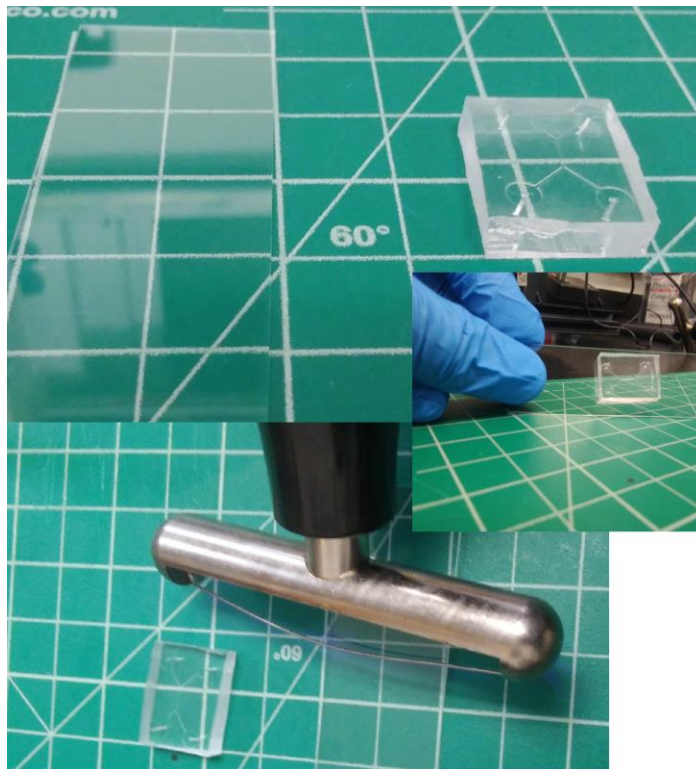
FIG. 5. Bonding the PDMS channel with glass.
