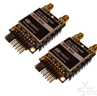
Figure VI. RFD 900X 900Mhz Telemetry Receiver
