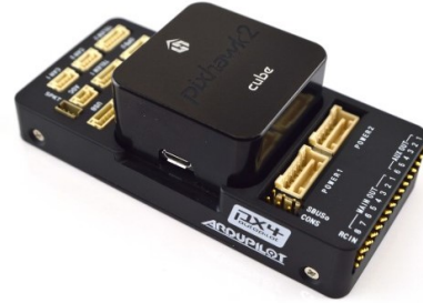
Figure XIX. Pixhawk 2.1 Cube Flight Controller
