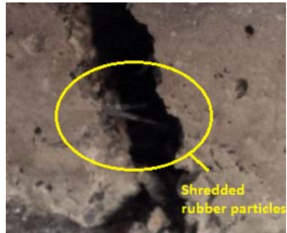
Fig. 5 Bridging of shredded rubber particles at crack
