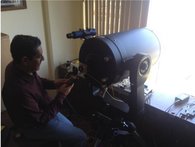
Fig. 3. User calibrating the telescope in the receiver side.
