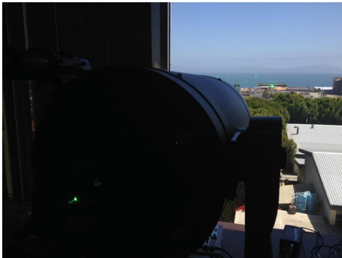
Fig. 4. Alignment process between the transmitter (bottom) and receiver (front) side using a green laser.
