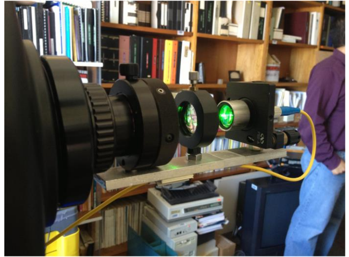
Fig. 5. Collimating set-up in the receiver side
