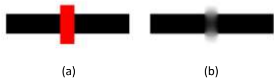
Figure 3. (a) An image of an edge with a hole, and (b) the same image reconstructed using the heat equation.
