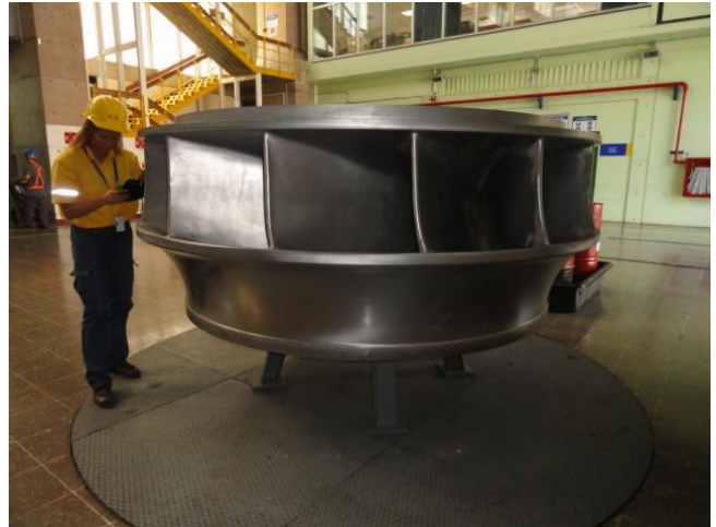
Fig. 1 Francis rotor of the Corobicí Project.
