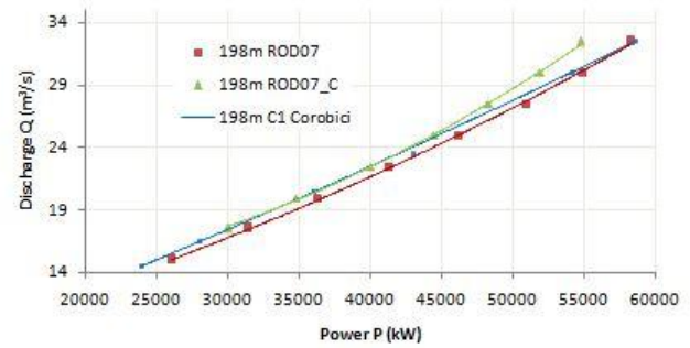
Fig. 5 Discharge curves of the real and simulated turbines.
