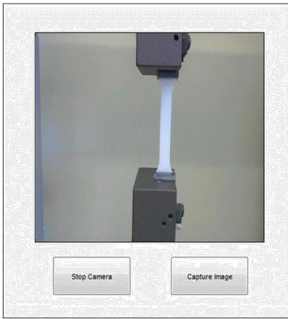
Fig.6: Camera Preview Window showing Nylon Specimen under Tensile Test
