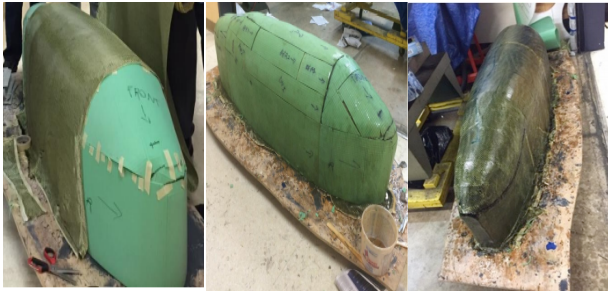
Fig 7: Three Step Process Laying Carbon-Kevlar Material
