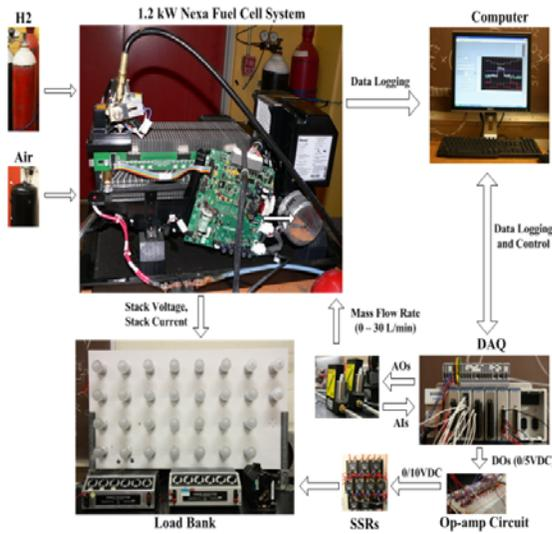
**Figure 2: Block diagram of FC experimental set-up and controller implementation**
