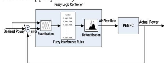
**Figure 3: Blok Diagramo f Fuzzy Logic Controller**
