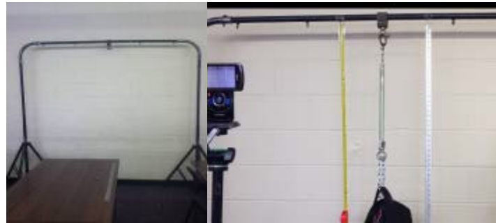
Figure 7: Stand, weighted bag and measuring tools used to suspend and test prototype device
