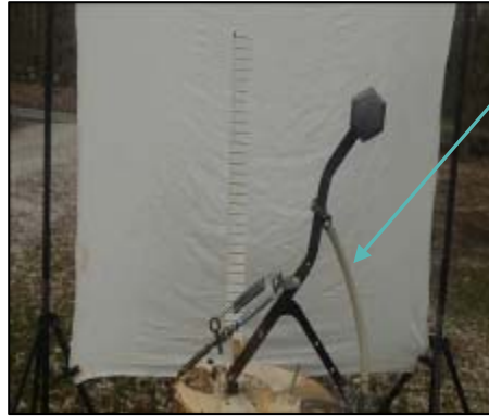
Figure 10: Physical experiment of idealized spine and head mass model
