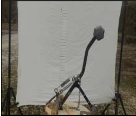
Figure 10: Physical experiment of idealized spine and head mass model
