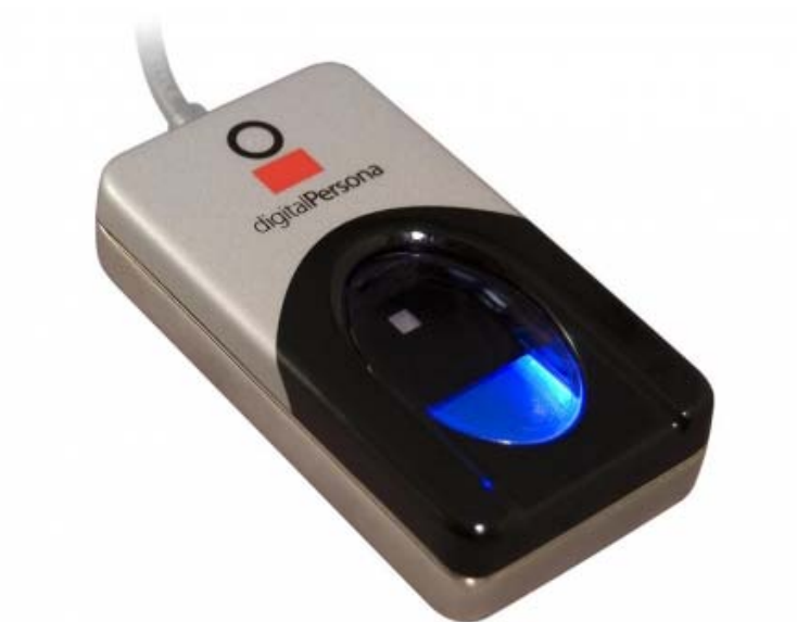
Figure 3. Reader Digital Persona fingerprint mark
