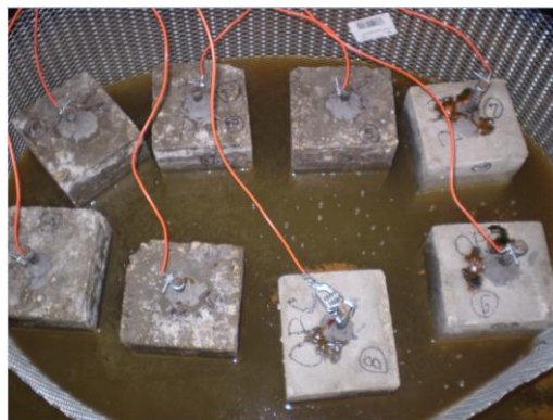
Figure 5: beams after 40 hours of accelerated corrosion testing 9 th Latin American and Caribbean Conference for Engineering and Technology
