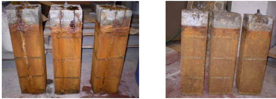
Figure 7: Physical appearance of OPC and GPC beams after accelerated durability testing
