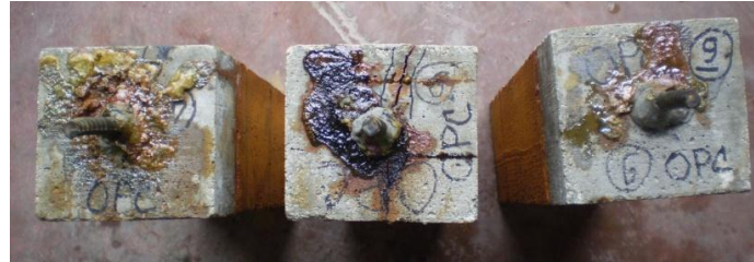
Figure 8: Top view of OPC beams shortly after accelerated durability testing (300 hrs)
