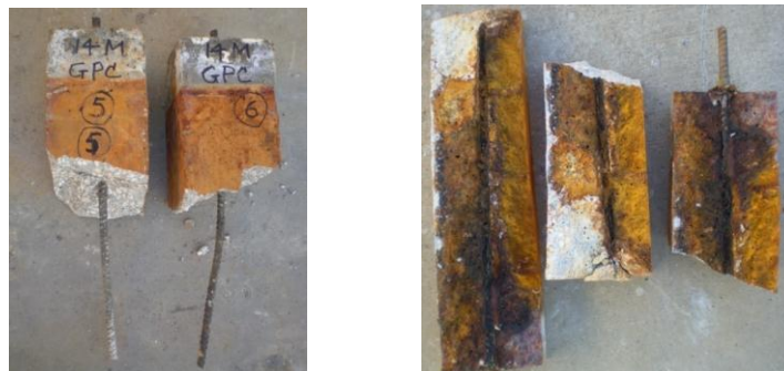
Figure 9: Broken OPC and GPC beams
