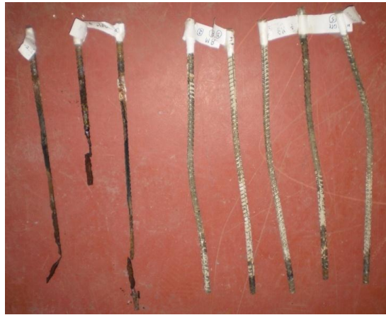
Figure 1: Retrieved rebars after accelerated corrosion testing
