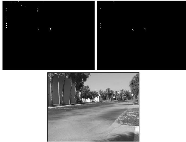
Figure 5: Grayscale image (bottom), background subtraction algorithm (top-left), and morphological filter output (top-right).
