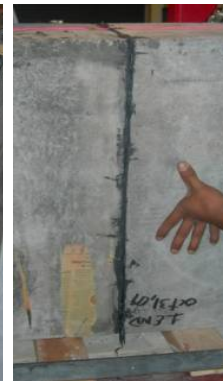
c) Jacking of central strand P1 and joint closing
