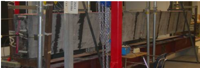
b) Full postensioned segmental beam and final alignment error of 3/4" (Length/340)
