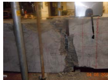
b) Central segment after failure
