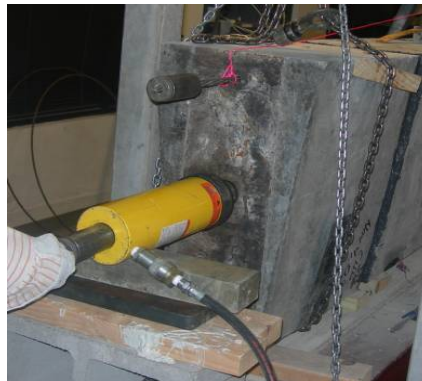
c) Jacking of central strand P1 and joint closing
