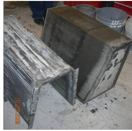
b) Concrete pouring and segment after form removal
