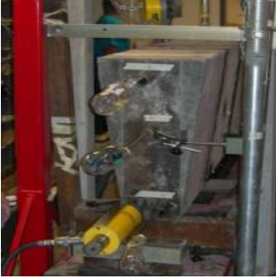
a) Sequence of postensioning after the beam was positioned on its supports: Strand P2 until 28 kips, Strand P3 until 15 kips, and Strand P4 until 28 kips
