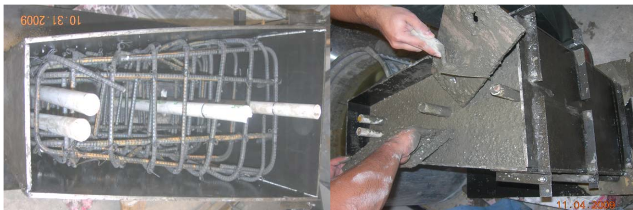
a) Anchor steel plate, pipes to install the strands, and rebar inside the form (2.2 in 2 vert., 3.3 in 2 hor., and 1.32 in 2 long.) b) Concrete pouring verifying that the pipes are in the correct position.
