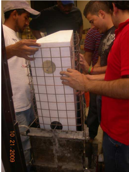
a. Preparing the steel mold and the foam block
