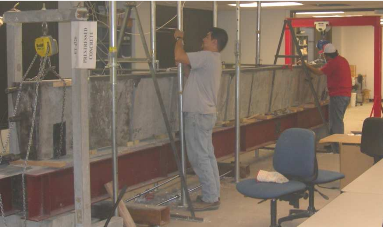
Figure 7. High-Strength Lightweight Concrete Segmental beam constructed over the testing beam
