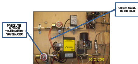
Figure 3. Sensors and transducers integration board (Fuel Cells Laboratory @ FAU)
